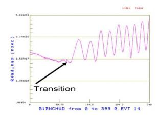
Figure 7: After implementing the radial motion at transition, the Booster  $4\sigma$  of bunch length at beam intensity of 5e12 ppp.
