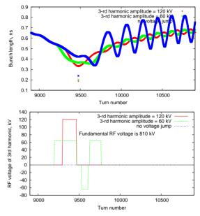
Figure 4: Bunch length (top) and 3-rd harmonic of rf voltage (bottom) at the Booster intensity of 5e12 ppp for three cases: voltage jump with 3-rd harmonic amplitude of 120 kV (red), with 3-rd harmonic amplitude of 60 kV (green) and without voltage jump (blue).
