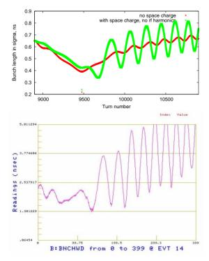
Figure 3: The  $\sigma$  of bunch length vs turn number in simulations at the beam intensity of 5e12 ppp, without (red) and with (green) space charge effect (top), and measured in the Booster  $4\sigma$  of bunch length (bottom).
