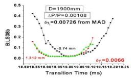
Figure 2: The beam loss at transition for two radial positions of the beam: 1.31mm (red and green) and -0.74mm (black).
