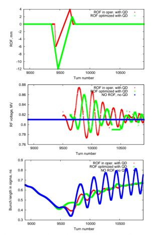
Figure 6: The radial motion (top), rf voltage (middle), and bunch length (bottom) at beam intensity of 4.5e12 ppp for three cases: with operational radial motion and the quad damper on (red); with optimal radial motion and quad damper on (green); and without any radial motion and quad damper off (blue).
