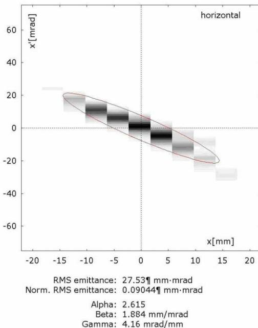
Figure 7: Horizontal phase space plot of the  $^{129}\text{Xe}^{14+}$  ion beam.
