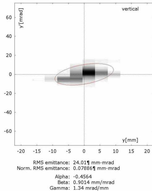
Figure 8: Vertical phase space plot for the  $^{129}\text{Xe}^{14+}$  ion beam.
