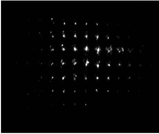
Figure 6: Pepper pot image of  $^{129}\text{Xe}^{14+}$  ion beam.
