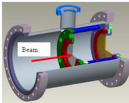
Figure 5: Cut-out view of the pepper pot – scintillator screen assembly.
