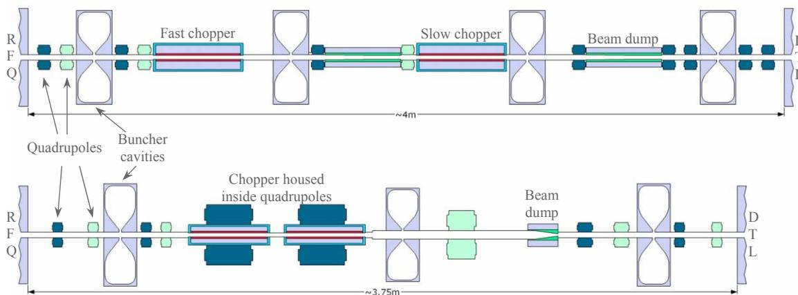
Figure 1: Schematic drawing of the RAL Scheme A (top) and the CERN MEBT Line (bottom).
