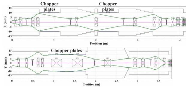
Figure 2: MEBT Beam Envelopes (from Partran, 5 RMS) in the chopping plane for RAL (top) and CERN (bottom) with the beam chopper switched off.
