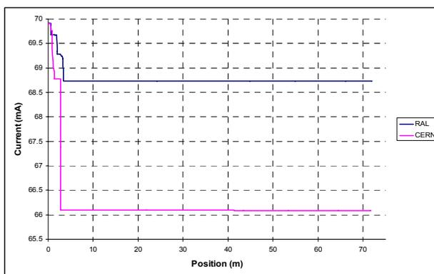
Figure 4: Beam current variation in LINAC4 using RAL and CERN MEBT lines.
