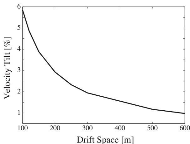
Figure 6: Required head-to-tail velocity tilt for the twice compression of the pulse duration as a function of the drift space.
