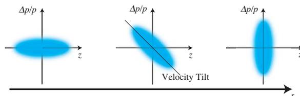
Figure 5: Bunch compression scenario with a head-to-tail velocity tilt in a phase space of a momentum spread  $\Delta p/p$  and a longitudinal direction  $z$  along the transport distance  $s$ .
