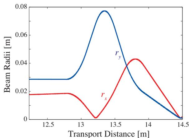
Figure 4: Beam envelope including the space charge effect around the focal position.
