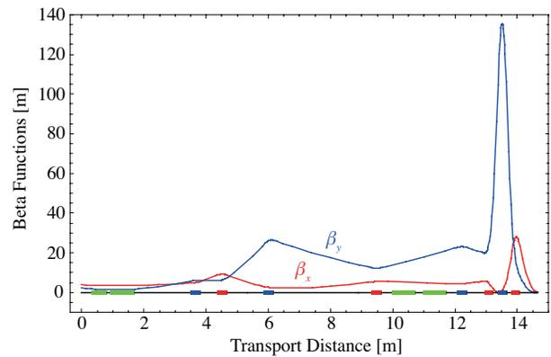
Figure 3: Beta functions and lattice components in the focus line for WDM experiments.
