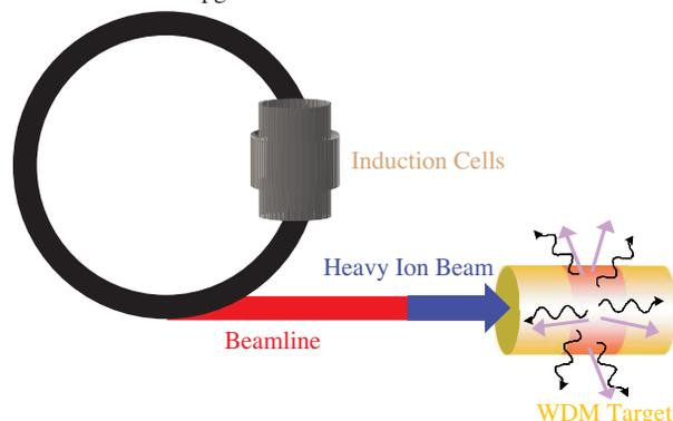
Figure 1: Outline of the 500 MeV Booster improved as the AIA and the beamline for the WDM experiment.
