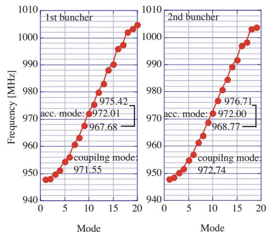
Figure 2: Plots of the dispersion curve.
