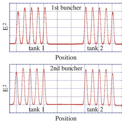
Figure 3: Electric field distribution.
