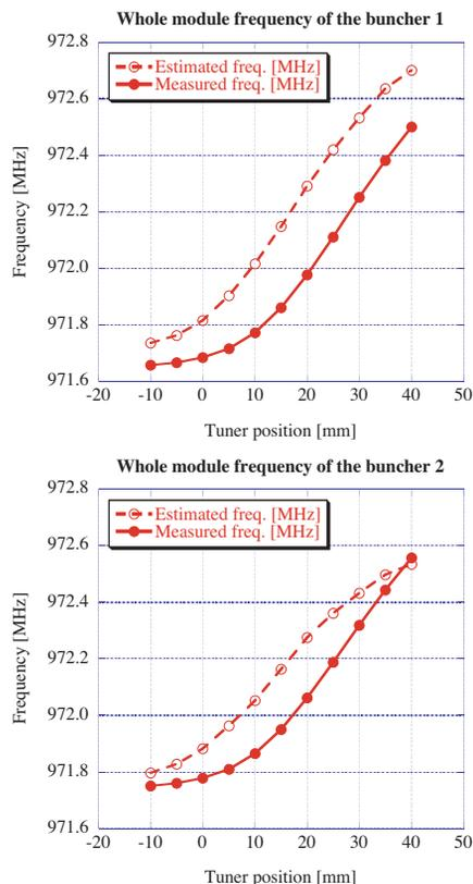
Figure 4: Estimated whole module frequency vs. measured frequency.
