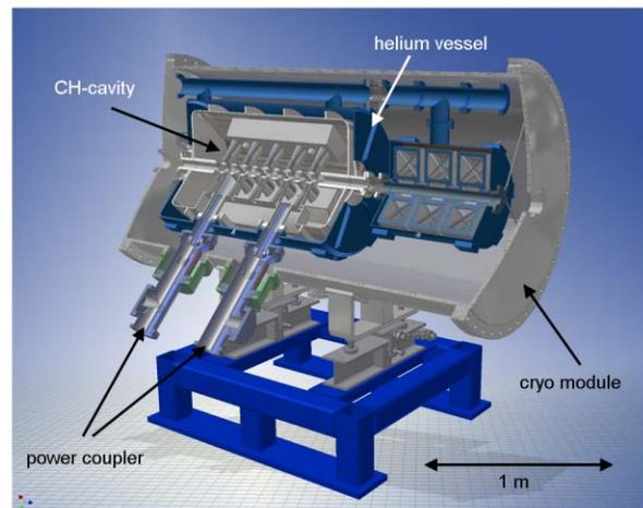
Figure 4: Cryo-module for the EVEDA-test with the first s.c. CH-cavity and two power couplers.
