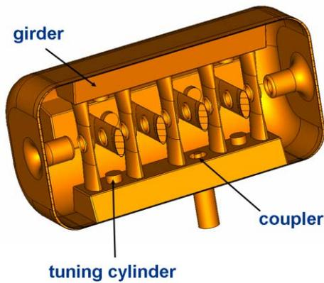
Figure 5: Model of the first s.c. CH-cavity.
