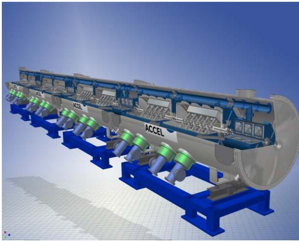
Figure 2: Study of the superconducting CH-linac for IFMIF. Eight cavities are housed in one modular cryo-module. Each cavity is fed by two 250 kW coaxial power couplers.
