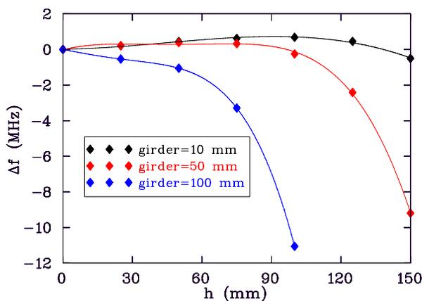
Figure 6: Frequency shift as function of the height of the foreseen tuning cylinders.
