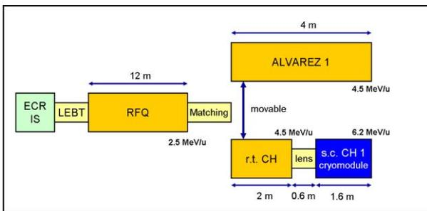
Figure 3: Possible test setup to test both the reference as well as the superconducting solution.
