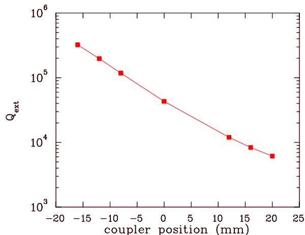
Figure 7: Simulated external Q-value as function of the coupler position. Due to the high beam current an external Q-value of 10<sup>4</sup> is required for each coupler.
