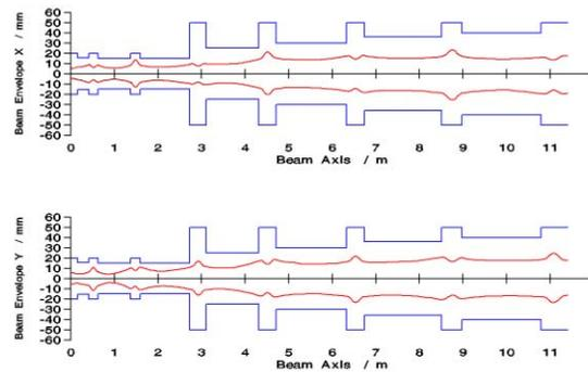
Figure 8: Plot of the transverse 100% envelopes along the proposed IFMIF-linac (without errors).
