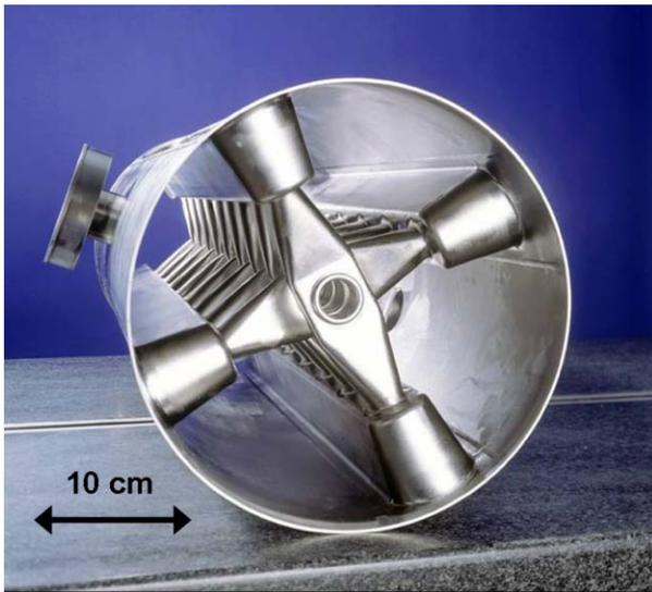
Figure 1: The superconducting CH-structure developed at IAP in Frankfurt. The prototype cavity has 19 accelerating cells, the geometrical  $\beta$  is 0.1. The cavity has been tested successfully at the cryogenic laboratory in Frankfurt (AC-CEL GmbH).
