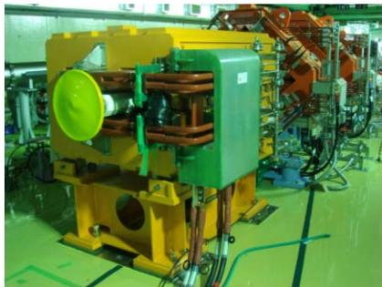
Figure 2: The pulsed bending magnet installed in the 3-50 BT tunnel.
