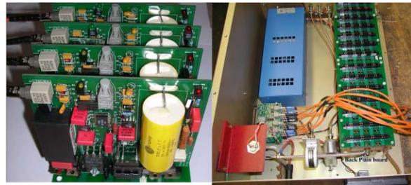
Figure 4: Prototype modulator drivers and motherboard
