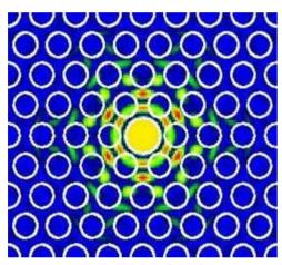
Figure 5: Increased accelerating field for a 1  $\mu m$  mode in a modified Lin fiber.
