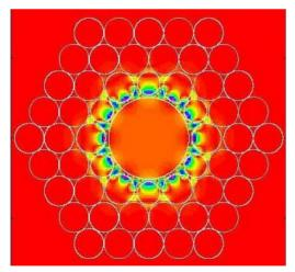
Figure 2: Accelerating field intensity of a 1.89  $\mu$ m mode in a circular-hole model of the HC-1550-02 fiber as calculated with CUDOS. To accent the weak fields in the core, an inverted color scale is used with blue being the highest field and red the lowest.
