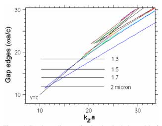
Figure 4: Band gap diagram for the circular-hole model of the HC-1550-02 fiber from R-Soft BandSolve. For reference, some free-space wavelengths are shown for a lattice hole spacing of  $3.8 \mu m$ .
