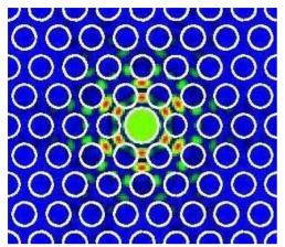
Figure 1: Accelerating field intensity of a 1  $\mu$ m mode in a Lin fiber as calculated with CUDOS. The longitudinal direction is out of the page. The color scale is relative with red being the highest field and blue the lowest.
