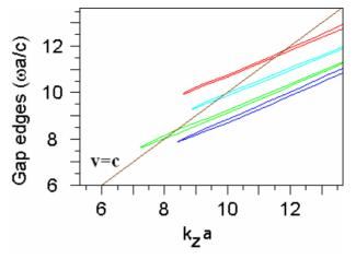
Figure 3: Band gap diagram with SOL line indicated for the Lin fiber as calculated with R-Soft BandSolve.
