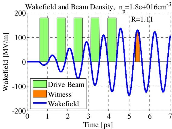
Figure 1: (Max Wakefield Scheme) Bunch distribution for maximum wake generation. A witness bunch  $180^\circ$  out of phase samples the accelerating wakefield.
