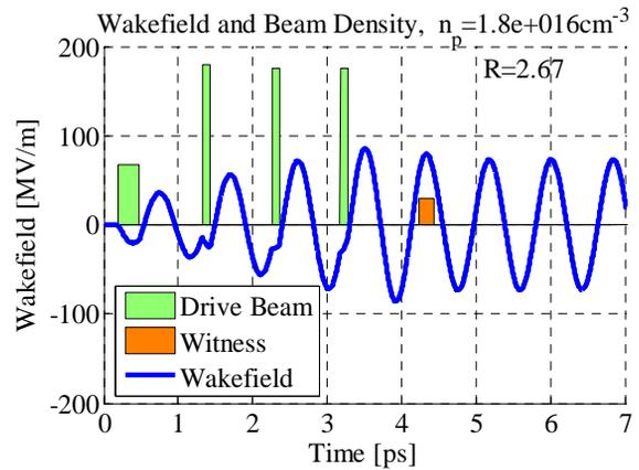
Figure 3: (Phased Bunch Scheme) Four bunches with equal charge placed properly (Eq.4) enhance the transformer ratio beyond 2.
