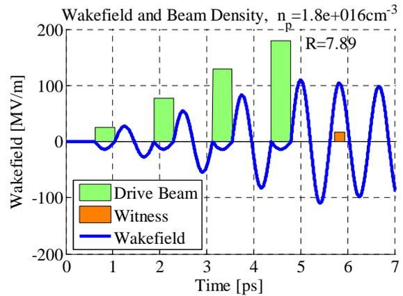
Figure 2: (Ramped Bunch Train Scheme) Bunch distribution for maximum transformer ratio. The drive bunches are separated by 1.5 plasma wavelengths.
