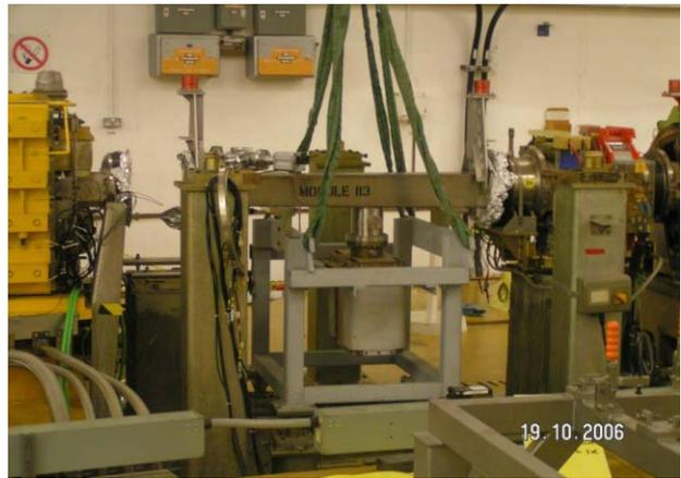
Figure 4: Plunging target mechanism in the ISIS ring.
