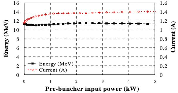
Figure 4: Output beam energy and current vs. input RF power into pre-buncher.
