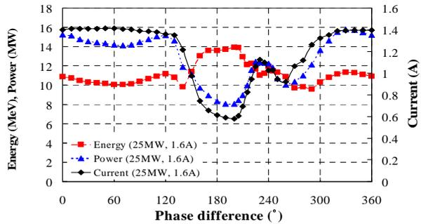
Figure 5: Output beam energy, power and current vs. input RF phase difference.
