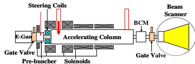
Figure 1: Schematic of the beamline of the L-band electron linac.
