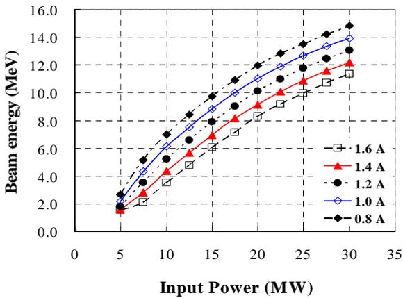
Figure 3: Beam energy vs. input RF power into the accelerating column.
