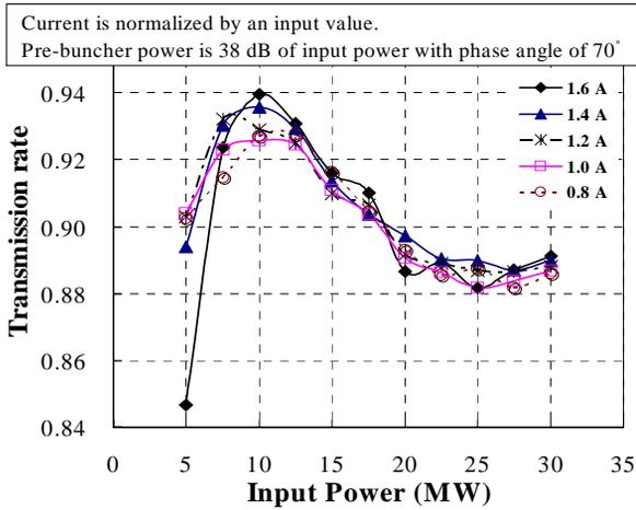
Figure 2: Beam transmission vs. input RF power into the accelerating column.
