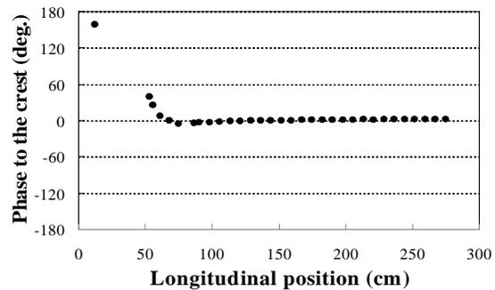
Figure 6: Variation of beam phase relative to crest of the wave through the beamline at the 330° phase difference.
