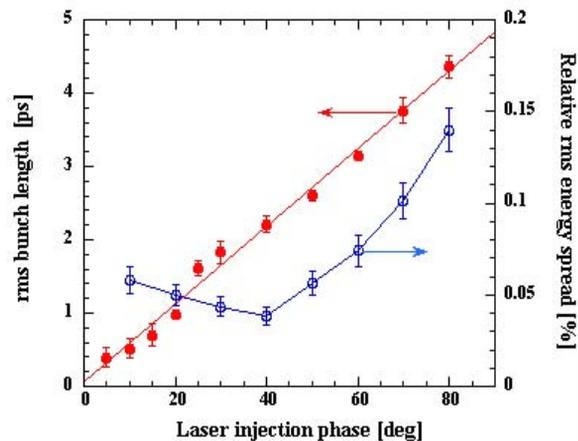
Fig. 3 Energy spread and bunch length versus laser injection phase
