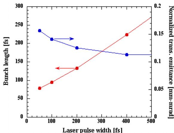
Fig. 6 Bunch length and transverse emittance versus incident laser pulse width
