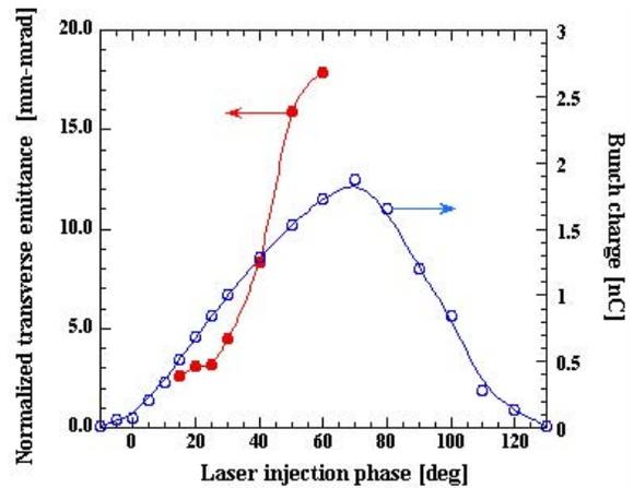
Fig. 2 Transverse emittance versus laser injection phase
