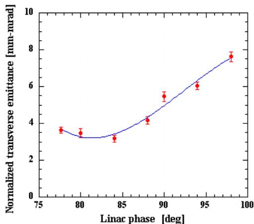
Fig. 4 Transverse emittance versus linac phase
