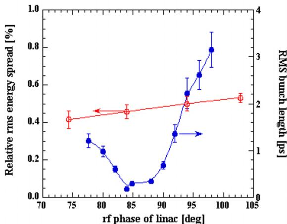
Fig. 5 Energy spread and bunch length versus linac phase
