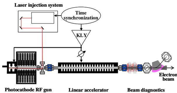
Fig. 1 The ultrashort-bunch electron linear accelerator
