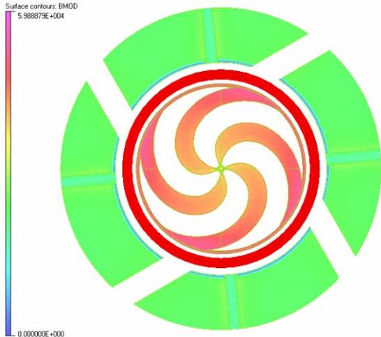
Figure 1: Top view of the magnetic field in the hills and the yoke.
