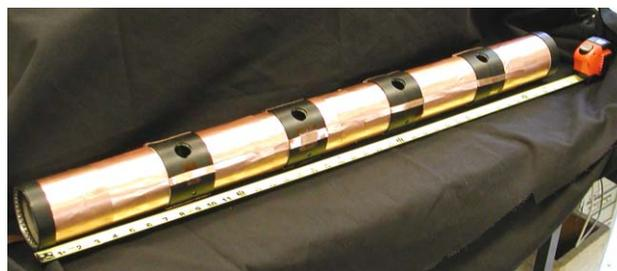
Figure 1: The one-meter-long BaTiO<sub>3</sub> FEPS consists of five individual sources with diagnostic ports between the sources.
