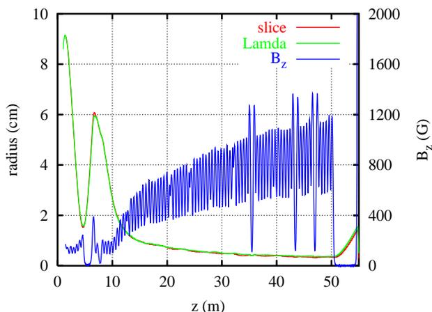
Figure 2: Comparison of the LSP slice algorithm and envelope code LAMDA. The beam edge radius is shown as a function of  $z$  for the entire length of the DARHT-2 accelerator. The on-axis magnetic field for the slice simulations is also shown.
