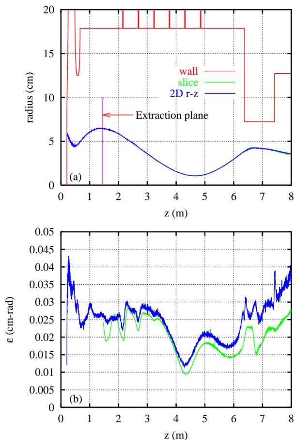
Figure 1: Comparison of slice algorithm and full 2-D  $r - z$  LSP simulation of the DARHT-2 injector. The diode voltage is 2.5 MV and the beam current is 2 kA. (a) Edge radius and (b) normalized edge emittance as a function of  $z$  are shown.
