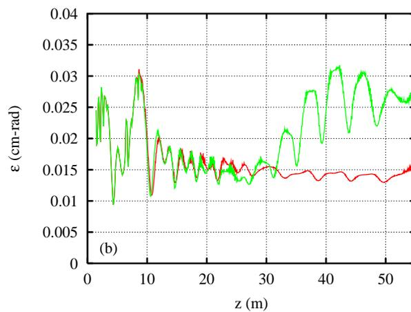
Figure 3: Comparison of edge radius and emittance for matched and mismatched transport. In the mismatched case the current applied to the solenoid centered at  $z = 8.2$  m is increased by 15 %.
