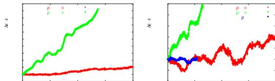
Figure 1: Emittance growth simulated with TAILHEAD considering a single electron-beam interaction point at the center of each half cell (left) and with two interaction points, close to the QD and QF quadrupoles (right). The electron cloud responds either dynamically, or it is frozen. The electron density is  $2.75 \times 10^{11} \text{ m}^{-3}$  for the left picture and either  $1 \times 10^{11} \text{ m}^{-3}$  or  $2 \times 10^{11} \text{ m}^{-3}$  on the right.
