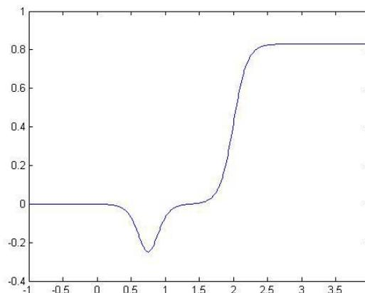
Figure 1. Magnetic field as a function of  $z$  in a magnetic system with inverse pole.
