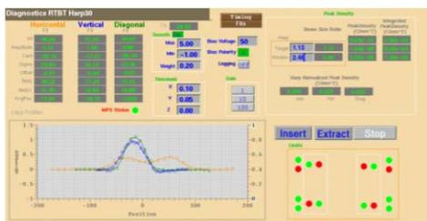
Figure 6: The harp screen with peak density values.
