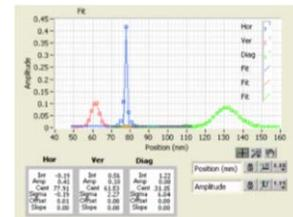
Figure 7: First profiles of new wire scanner application.
