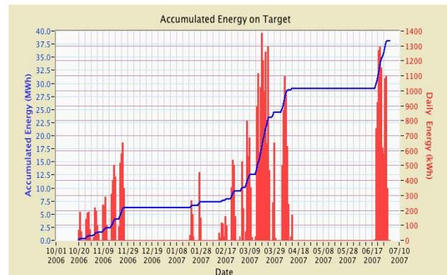
Figure 5: Integrated beam power (kW-hrs) delivered per day. The blue curve shows the cumulative quantity (MW-hrs) since the beginning of the fiscal year.
