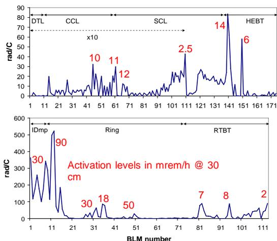
Figure 6: Beamloss (rad/C) plotted vs. beam loss monitor number in the linac (top) and ring (bottom). The activation levels in mrem/hr at 1 ft after 30 hour cooldown are shown in red.
