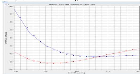
Figure 1: Results of phase-scan signature matching to determine RF setpoints. BPM phase difference is plotted vs. DTL tank 4 phase. The curves show data for two RF amplitudes. The points show the results of model-based fitting.
