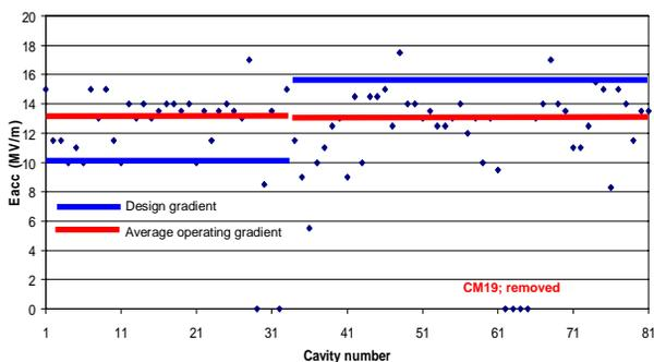
Figure 2: Accelerating gradient vs. cavity number for the SCL.
