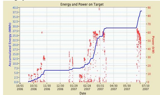
Figure 4: History of beam power delivered to the target since the beginning of formal SNS operations.
