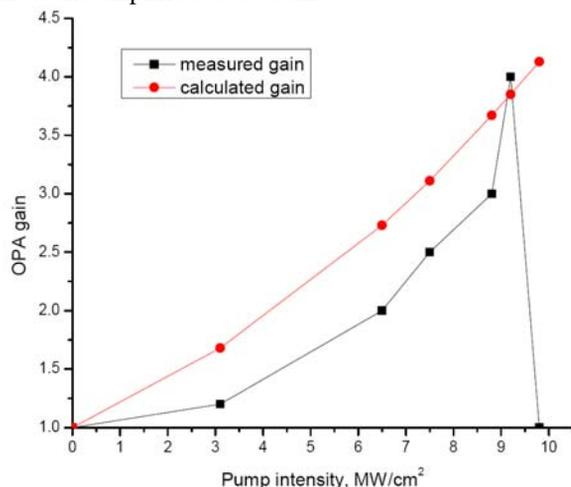
Figure 4: Measured (black) and calculated (red) dependence of the OPA gain upon the pump intensity.
