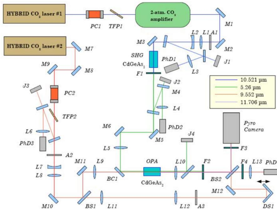
Figure 2: Layout of the OPA setup. Refer text for details.
