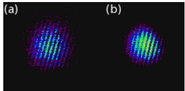
Figure 3: Interference pattern of non-amplified (a) and amplified (b) beam (at gain equal to 4.0)
