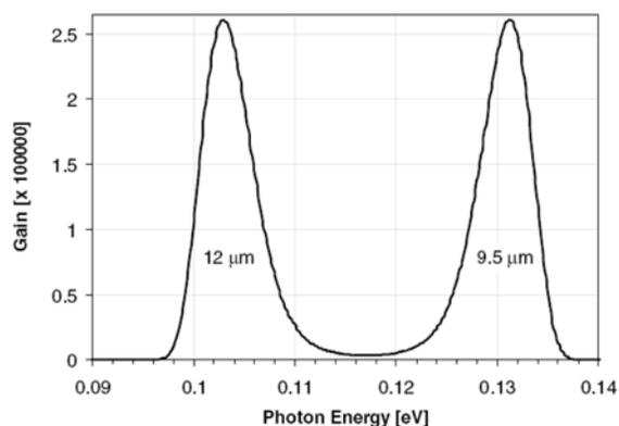
Figure 1: Dependence of the OPA gain on the photon energy of amplified radiation calculated using formulae from [5]
