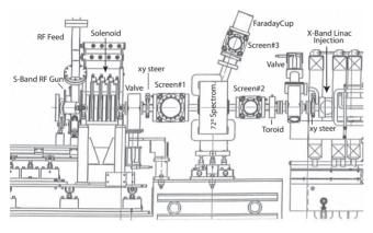
Figure 1: Layout of the SLAC NLCTA RF photoinjector.
