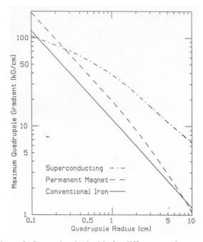
Figure 3: Strengths obtainable for different quads types[5]: iron pole-tip fields  $B_p=12$  kG, remanent fields  $B_r=11.5$  kG for PMs and NbTi wire with  $J_c=2$  kA/mm<sup>2</sup> at 5T & 4.2°.
