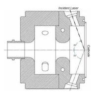
Figure 2: Schematic, cross-sectional view of a 1.6-cell, laser-driven RF gun. The internal, unshaded areas are to be maintained continuously at very high vacuum to sustain a stable and acceptable quantum efficiency as well as avoid RF breakdown damage. L or S-Band RF cells set the scale.
