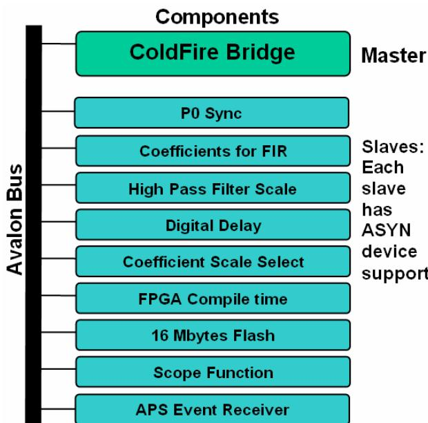
Figure 2: Avalon Bus components for P0 Feedback system.
