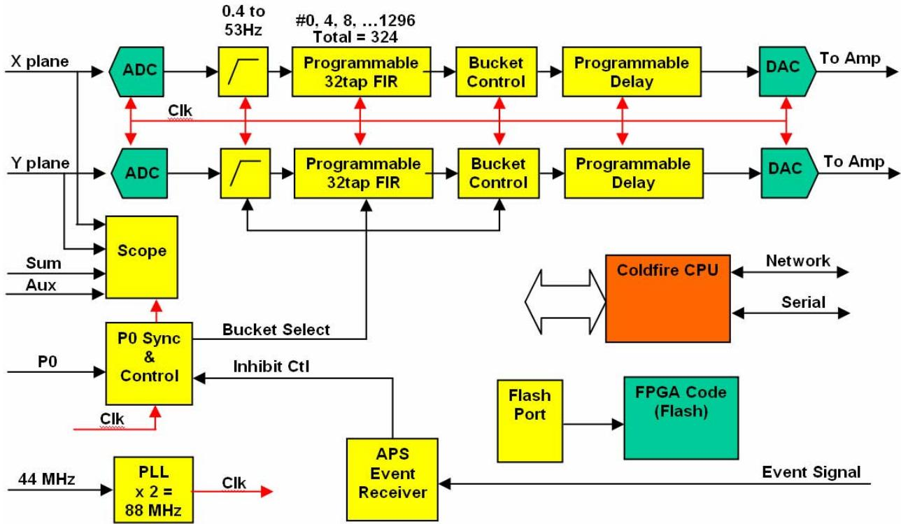
Figure 1: Block diagram of the P0 Feedback system.
