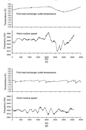
Figure 1: (A) The variations for first heat exchanger outlet temperature without  $LN_2$  pre-cooling, (B) The variations for first heat exchanger outlet temperature with 120K  $LN_2$  pre-cooling
