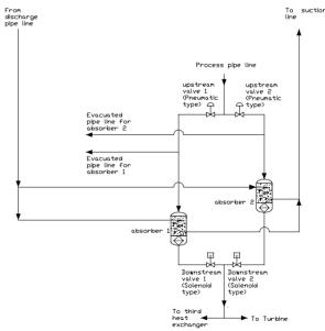
Figure 3 Schematic of pipeline for two 80K auto switched absorbers.
