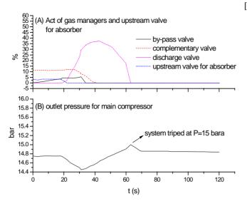
Figure 4 (A) The actions of gas managers and upstream valve for absorber, (B) Variation of outlet pressure for main compressor
