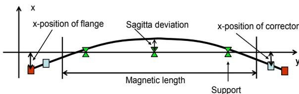
Figure 3: The sagitta change of an assembled magnet changes also the position of the correctors and the flanges. The magnets were blocked at the central support to avoid the shape-change.
