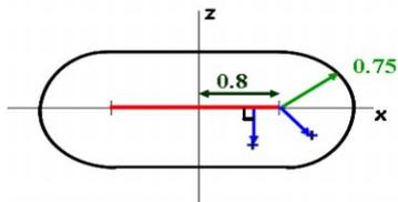
Figure 2: Tolerances for the dipole. The tolerances define the “silver” class, represented here in a plane perpendicular to the magnet axis: the cross is the position of the beam tube centre and it has to lie within the race-track shape. Dimensions in mm.
