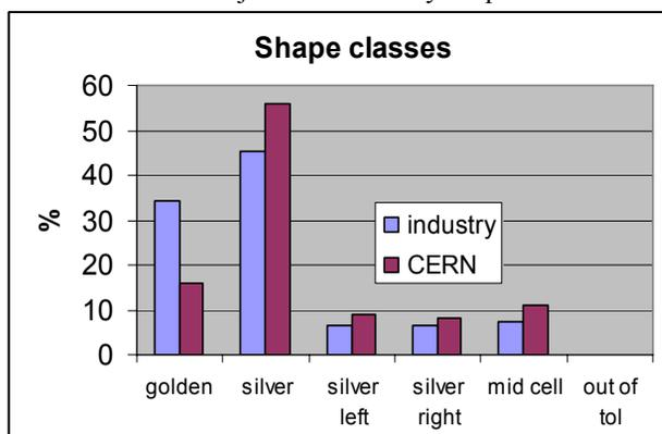
Figure 4: Magnet shapes in industry and after last measurement at CERN.
