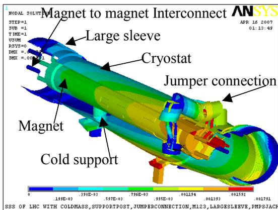
Figure 1: A view of the Short Straight Section Model.
