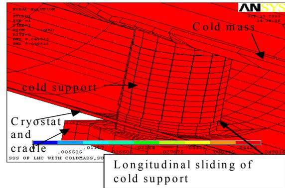
Figure 3: Cold Support and the sliding behaviour in longitudinal direction.
