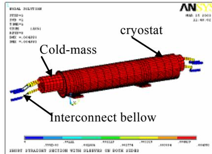
Figure 6: FE model of magnet to magnet interconnects.
