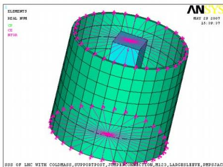
Figure 2: FE model of Cold support.
