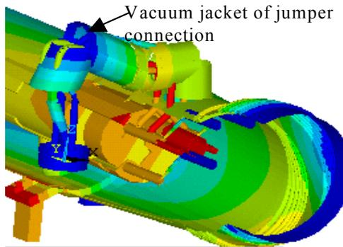
Figure 4: FE model of the Jumper Vacuum jacket.
