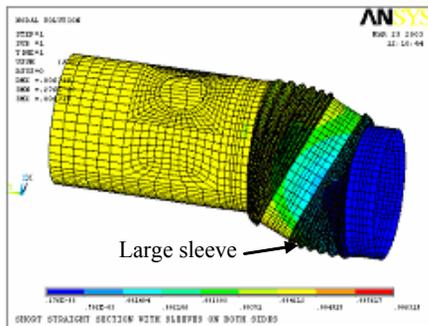
Figure 5: FE model of large sleeve.
