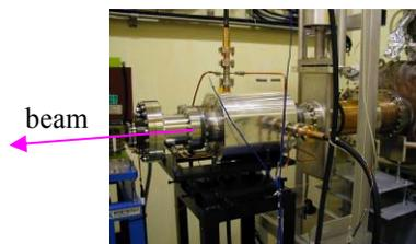
Figure 1: Drawing and a photo of the longitudinal kicker installed at downstream of the RF accelerating cavity. Blue cables in the photo are temperature sensors.
