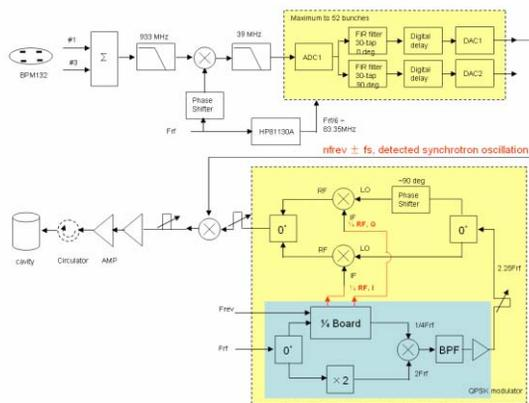
Figure 5: Bunch-by-bunch feedback system using Xilinx FPGA evaluation board and QPSK modulator.
