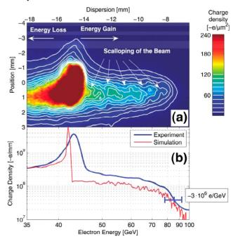
Figure 1. (a) The energy spectrum of the (initially nominally 42 GeV) electron beam after passage through an 85 cm long,  $2.7 \times 10^{17}$  cm<sup>-3</sup> Lithium plasma and (b) a comparison between the measured spectrum and the simulated spectrum. Reprinted by permission from Macmillan Publishers Ltd: *Nature* 445, 741-744, © 2007.
