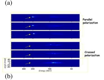
Figure 3. (a) Schematic set-up for controlling the injection of electrons in the wakefield by colliding a pump beam with an injection beam and (b) electron spectra obtained with the pump and the probe beam having parallel polarizations (top three events) and orthogonal polarizations (bottom three events). Only when the polarizations are parallel, a well defined monoenergetic beam can be seen as expected. Courtesy of V. Malka
