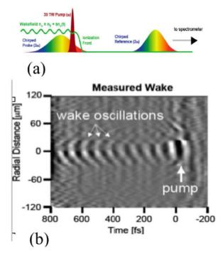
Figure 2. (a) Schematic of frequency domain holography and (b) the reconstructed hologram showing the wake oscillations obtained after Fourier transforming the frequency domain interferogram at the output of the spectrometer. Courtesy of M. Downer.
