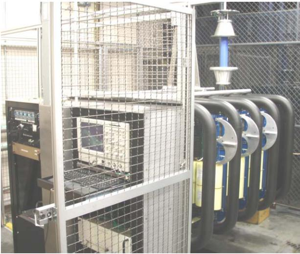
Figure 1: Photo of the SLAC Marx Modulator with 10 of the 18 cards installed.
