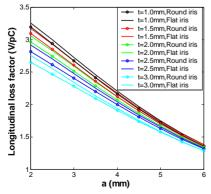
Figure 4: Comparison of the longitudinal loss factor for the structures with round edge and flat edge.
