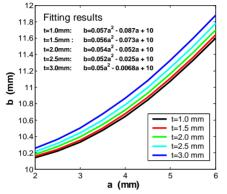
Figure 2: Relation between the aperture *a* and the radius *b* of a disc-load structure with round beam hole to maintain the accelerating mode frequency and phase constant.
