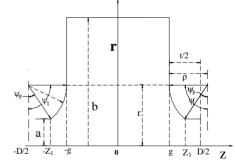
$\begin{array}{l} D = disk \ spacing \quad \rho = edge \ radius \quad r_c = radius \ of \ interface \\ t = 2(D/2 - g) = disk \ thickness \\ 2a = disk-hole \ diameter \quad 2b = inside \ cylinder \ diameter \\ 2\delta = 2(D/2 - Z_1) = flat \ land \ in \ disk \ hole \end{array}$
