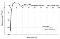
Figure 3: IR wake potential of a 0.25 mm bunch.
