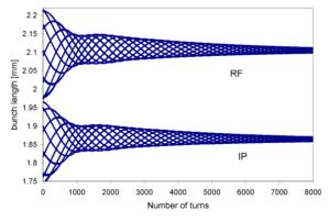
Figure 7: Bunch length in RF and IR.
