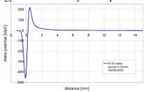
Figure 2: Resistive-wall wake potential of a 0.25mm bunch.
