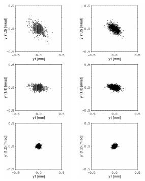
Figure 4: Vertical beam-centroid coordinates computed from data (left) and from simulation (right), for individual samples from first two BPMs (top), individual samples from first and last BPM (middle), and averaged data from first two BPMs (bottom).
