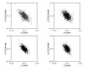
Figure 3: Horizontal beam-centroid coordinates computed from data (left) and from simulation (right), for individual samples (top) and averaged data (bottom) from first and second BPM.
