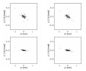
Figure 5: Vertical beam-centroid coordinates computed from data (left) and from simulation (right), for individual samples from first two BPMs (top) and from first and last BPM (bottom).
