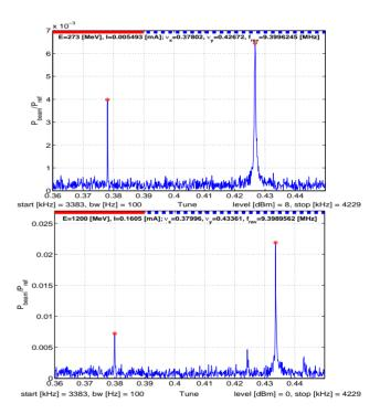
Figure 3: The measured betatron tune signals. The upper plot shows the measured tunes at the injection energy of 273 MeV with about 5  $\mu$ A of stored beam current; the lower plot shows the measured tunes at the highest extraction energy of 1.2 GeV with about 150  $\mu$ A of stored beam current.
