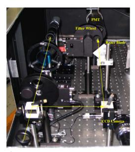
Figure 2: The optical detection system. The optical beam from a dipole synchrotron port passes a space filter (a razor blade) before being detected by a photomultiplier tube.
