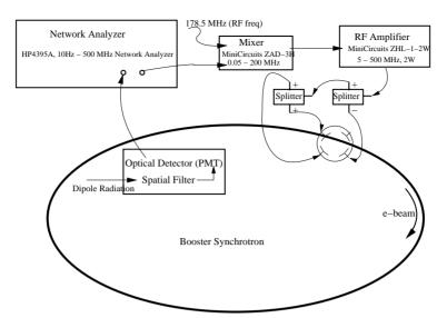
Figure 1: The layout of the booster scanning tune measurement system. A network analyzer excites the electron beam using a stripline BPM and the beam response signal is detected by an optical system with a space filter and a PMT.
