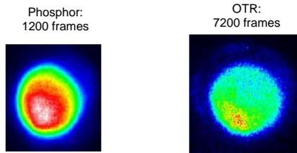
Figure 6: Comparison of phosphor screen and OTR images for a full 100 ns beam pulse; 100ns gate.
