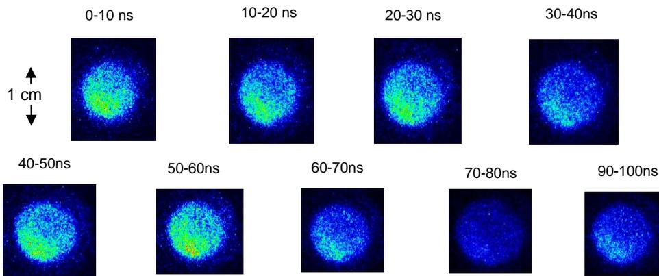
Figure 7: OTR images each taken with 7200 frames of 10ns gate duration, in progressive 10ns steps from the beginning to the end of UMER's 100 ns pulse.
