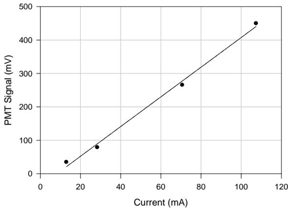
Figure 3: PMT signal as a function of beam current.
