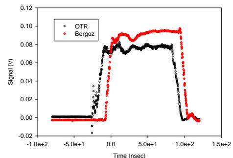
Figure 2: Comparison of PMT and Bergoz signals.
