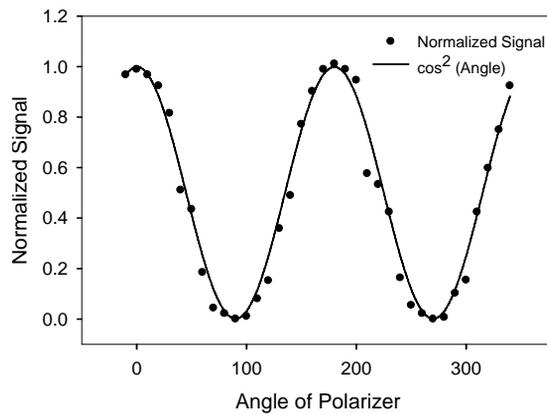
Figure 5: Radiation intensity measured as a function of polarizer angle with fit to a squared cosine distribution.
