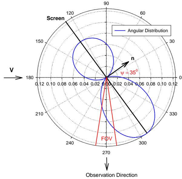
Figure 4: Theoretical angular distribution of OTR for a 10 keV ( $\beta = 0.139$ ) electron beam.
