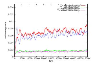
Figure 3: Horizontal and vertical emittance growth evolution of the blue beam with and without machine chromaticity at working point (0.714, 0.726) for 4 sigma separation.
