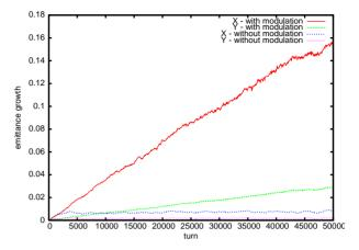
Figure 2: Horizontal and vertical emittance growth evolution of the blue beam with and without tune modulation at working point (0.714, 0.726) for 4 sigma separation.
