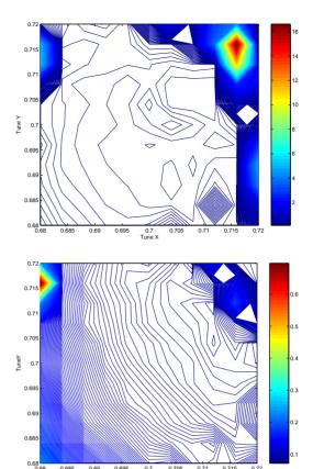
Figure 5: Averaged emittance growth as a function of betatron tunes for 4 sigma and 6 sigma separation including tune modulation.
