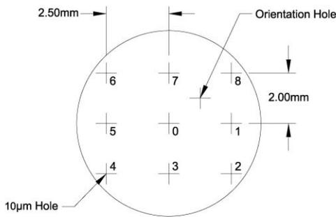
Figure 3: Pinhole Test Grid Layout (pinhole tol.: +/- 2 μm). Note: Reference orientation hole to account for optical image rotations induced.
