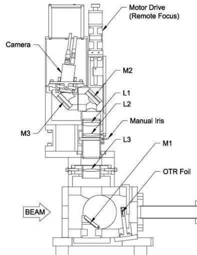
Figure 1: OTR-S1 assembly. The OTR foil is replaced with a pinhole array during laboratory bench testing.
