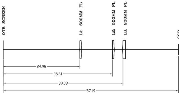
Figure 2: Nominal optical path configuration yielding a calculated optical resolution of approximately 10 μm with a 0.65 image demagnification.
