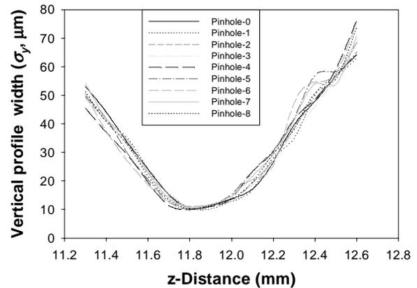
Figure 6: Gaussian widths of horizontal and vertical profiles of pinhole grid.
