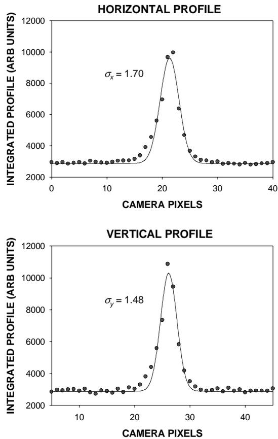
Figure 5: Integrated profile of the pinhole images in the horizontal direction (top profile) and vertical direction (bottom profile) fitted to Gaussian curves.
