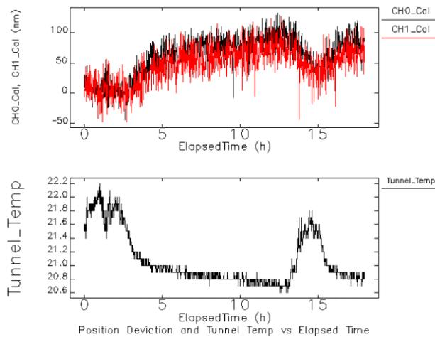
Figure 3: Electronics thermal stability test.
