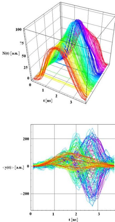
Figure 2: Longitudinal profile and vertical centroid position along the bunch. The head of the bunch is at  $t=0$ . The profiles are cut at  $\pm 3 \sigma_t$ .
