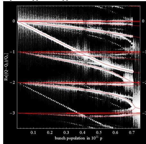
Figure 3: Head-tail modes vs. bunch intensity for  $\epsilon_L=0.2$  eV.s and  $\sigma_t=0.67$  ns,  $V_{RF}=0.6$  MV and  $\xi_v \sim 0$ . MOSES (red lines) vs. HEADTAIL (white dots whose size and brightness depend on the spectral amplitude) results analyzed with SUSSIX.  $Z_t=10$  M $\Omega$ /m,  $f_{res}=1$  GHz and  $Q=1$ .
