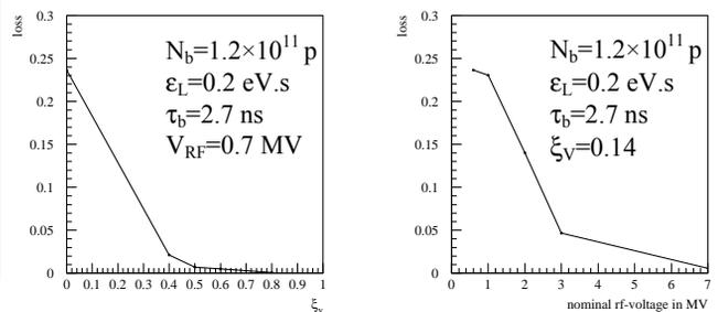
Figure 1: Fraction lost in the first 10 ms vs. vertical chromaticity (left) and capture RF voltage (right). The first point at low vertical chromaticity corresponds to ( $\xi_v=0.14$ ) while the first point at low RF voltage corresponds to  $V_{RF}=0.7$  MV.
