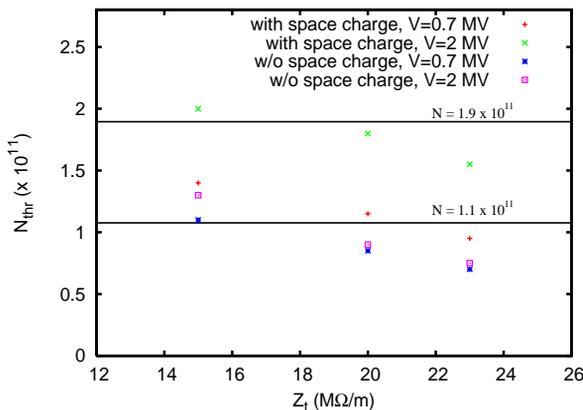
Figure 4: TMCI thresholds vs. broad-band shunt impedance for  $f_{res}=1$  GHz and  $Q=1$  for an LHC bunch.
