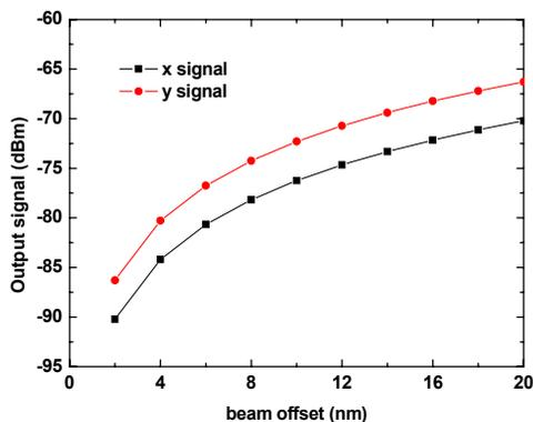
Figure 3: Calculated output signal vs. the beam offset.
