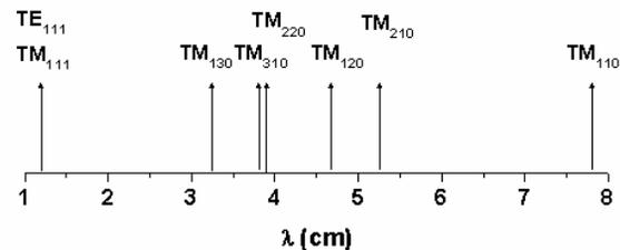
Figure 1: Mode spectrum of ATF IP-BPM. TM210 and TM120 indicate x dipole and y dipole modes, respectively.
