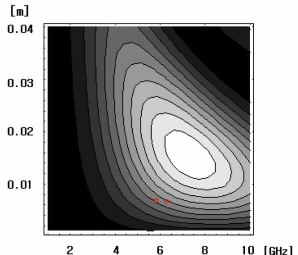
Figure 2: The generated dipole mode energy. Assumed bunch length is 8 mm rms. Marks of rectangular and circle indicate cases of x dipole and y dipole, respectively.
