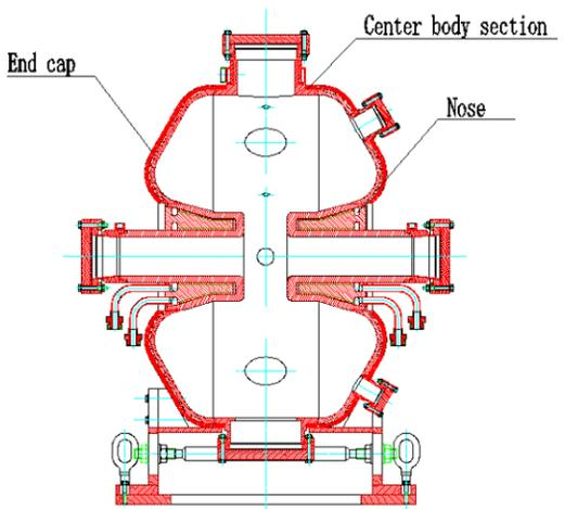
Figure 3: The sketch of HLS RF cavity.
