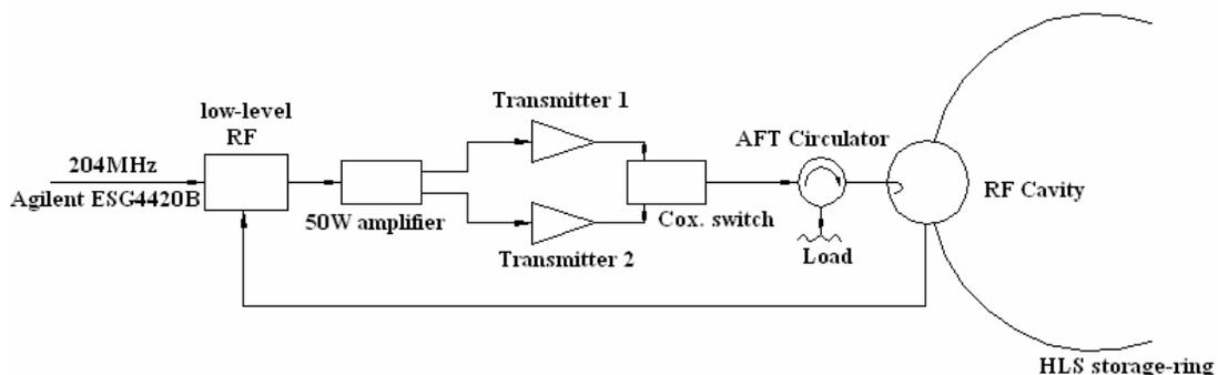
Figure 1: Block diagram of HLS RF system.
