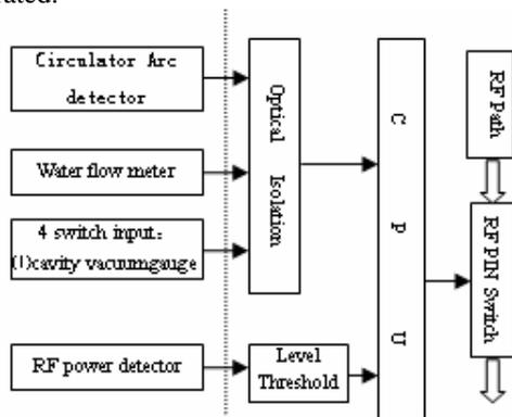
Figure 4: The Diagram of interlocks circuit.
