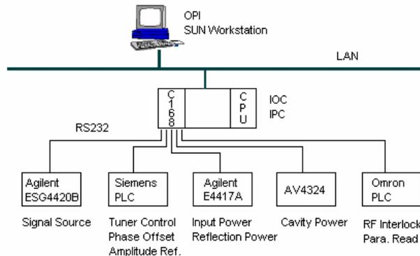
Figure 5: Hardware structure of HLS storage ring new RF control system.
