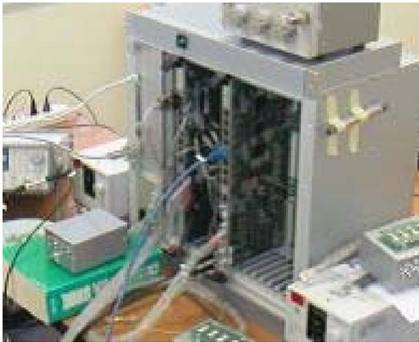
Figure 4: 9U VME chassis, SPG and RFG boards, under testing
