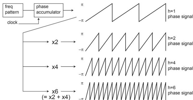
Figure 2: Direct Digital Synthesis (DDS)
