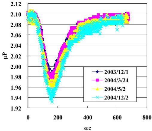
Figure 4: Changes of the dip depth of #14 klystron.
