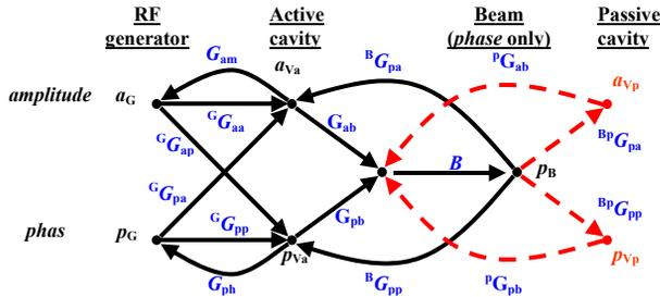
Figure 2: Signal-flow graph of the RF system.
