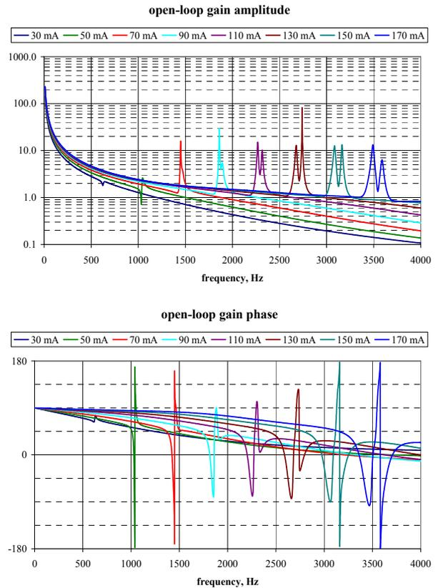
Figure 5: Open-loop Bode plot for different beam currents and the passive cavity parameters  $Q_{ext} = 2 \times 10^7$ ,  $V = 1.2$  MV.
