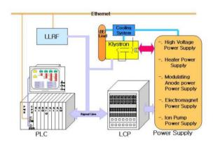
Figure 3 : Structure of sequence control system.
