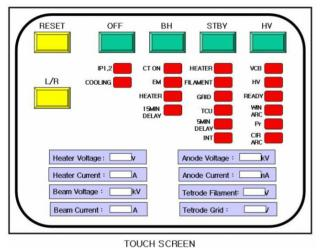
Figure 5: Configuration of touch screen.
