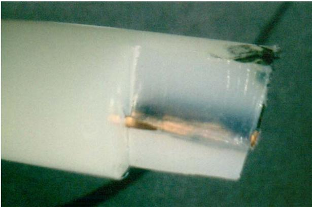
Figure 5: Damage of breakdown cable.
