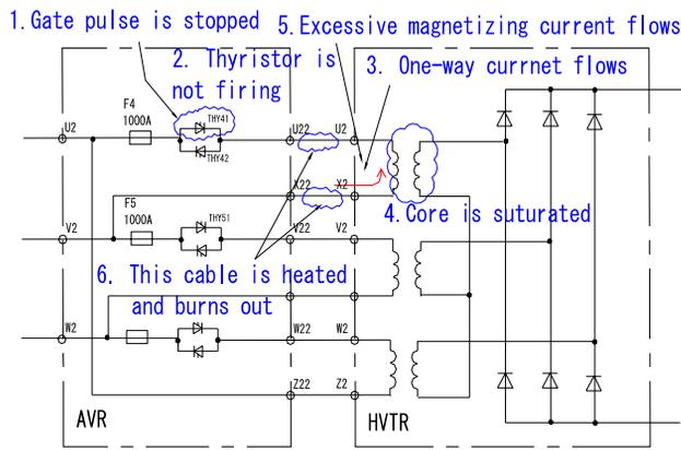
Figure 4: Illustration of the burned cable process.
