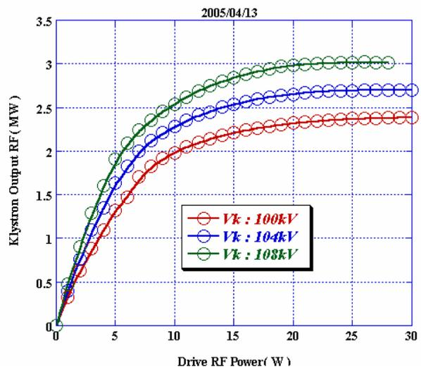
Figure 3: Characteristics of the 972MHz klystron.
