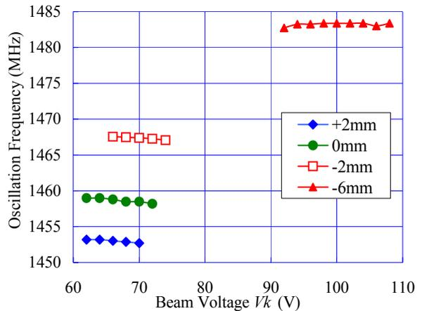
Figure 2: Dependence of oscillation frequency of mode C on deformation length in the 2nd cavity.
