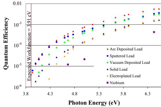
Figure 3: QE of lead cathodes at 1 MV/m applied field, after laser cleaning (0.2 mJ/mm<sup>2</sup>).
