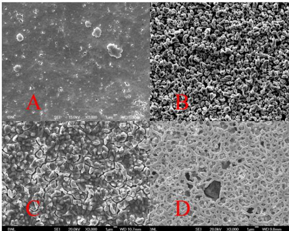
Figure 1: Surface structure of lead cathodes after laser irradiation with 0.2 mJ/mm<sup>2</sup>: (A) Arc deposited (B) Sputtered (C) Vacuum deposited (D) Solid lead.
