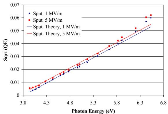
Figure 4: Sqrt QE vs photon energy for sputtered lead
