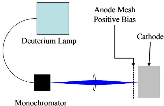
Figure 2: Apparatus for photoemission measurements.
