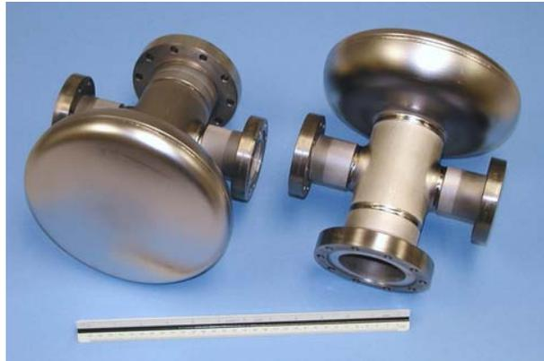
Figure 1: Photograph of 0.6 cell 1.3 GHz SRF cavity.
