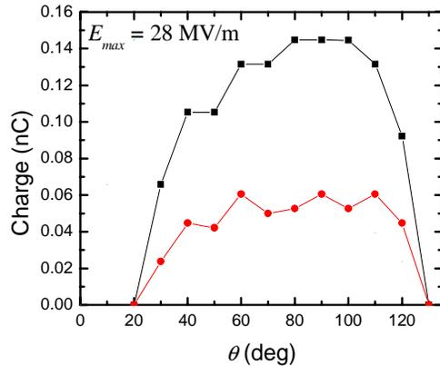
Figure 4: rf scans at  $E_{max} = 28$  MV/m for different laser intensities. No shift in the onset phase angle is detected. This shows that we are not close to the detection threshold.
