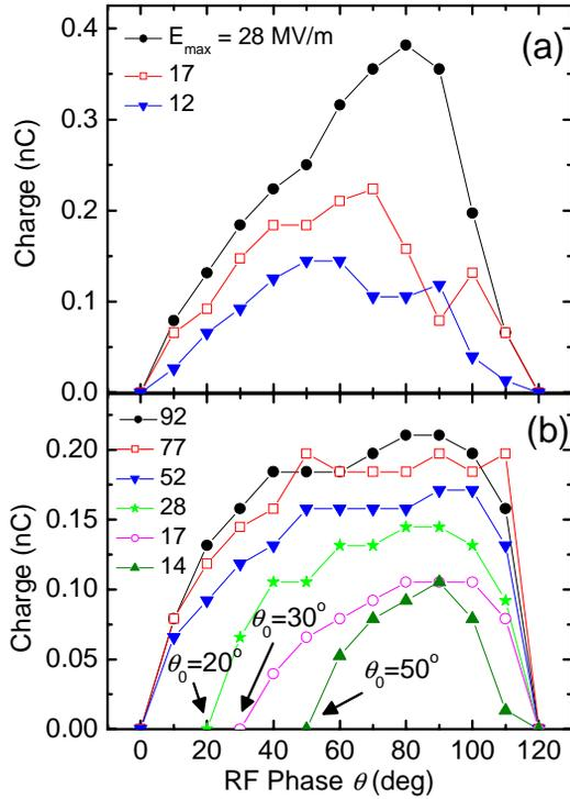
Figure 2: Charge emitted at various rf phase  $\theta$  from Mg cathode ( $\Phi_0 = 3.7$  eV). Electric field on the cathode is  $E(\theta) = -E_{max} \sin(\theta)$ . (a) Charge produced by 5 eV photons. (b) Charge produced by 3.3 eV photons.  $\theta_0$  is the phase angle ( $\pm 5^\circ$ ) at the threshold of photoemission.
