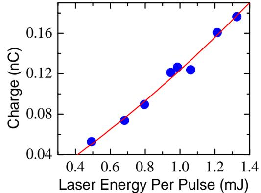
Figure 3: Charge vs. laser energy per pulse (intensity) from 3.3 eV photons. The solid line is approximately a linear fit. The electric field on the cathode is 70 MV/m.
