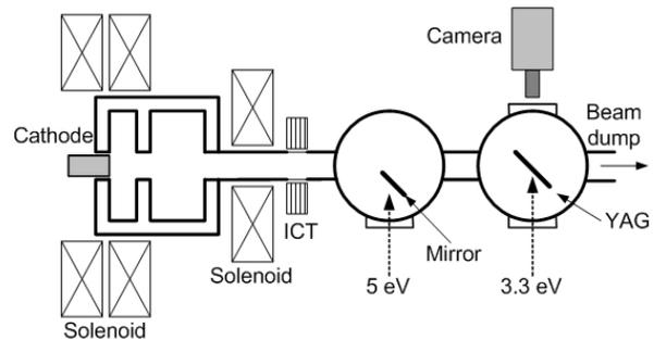
Figure 1: Schematic diagram of rf photoinjector. There are two laser input windows for different photon energies.
