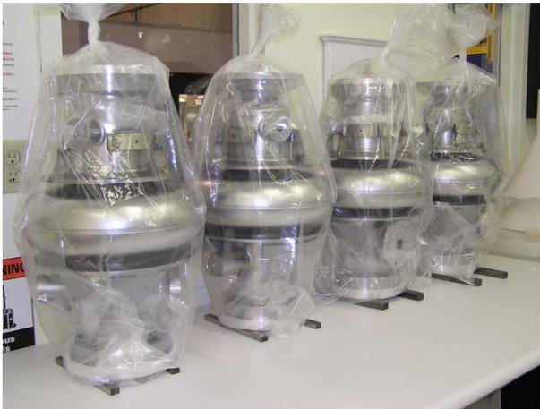
Figure 2: Four 748.5 MHz SRF fundamental cavities.
