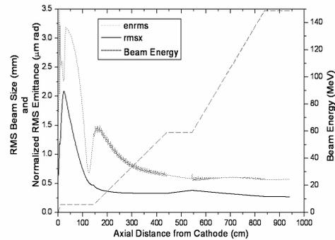
Figure 2. The beam size, emittance, and energy of our beam along the RF PC gun with the solenoid field profile is simulated by PARMELA code.
