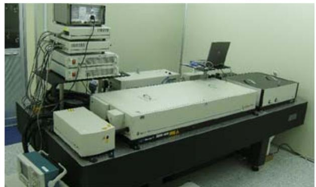
Figure 3. Ti:Sapphire laser system with 267nm wavelength is installed.
